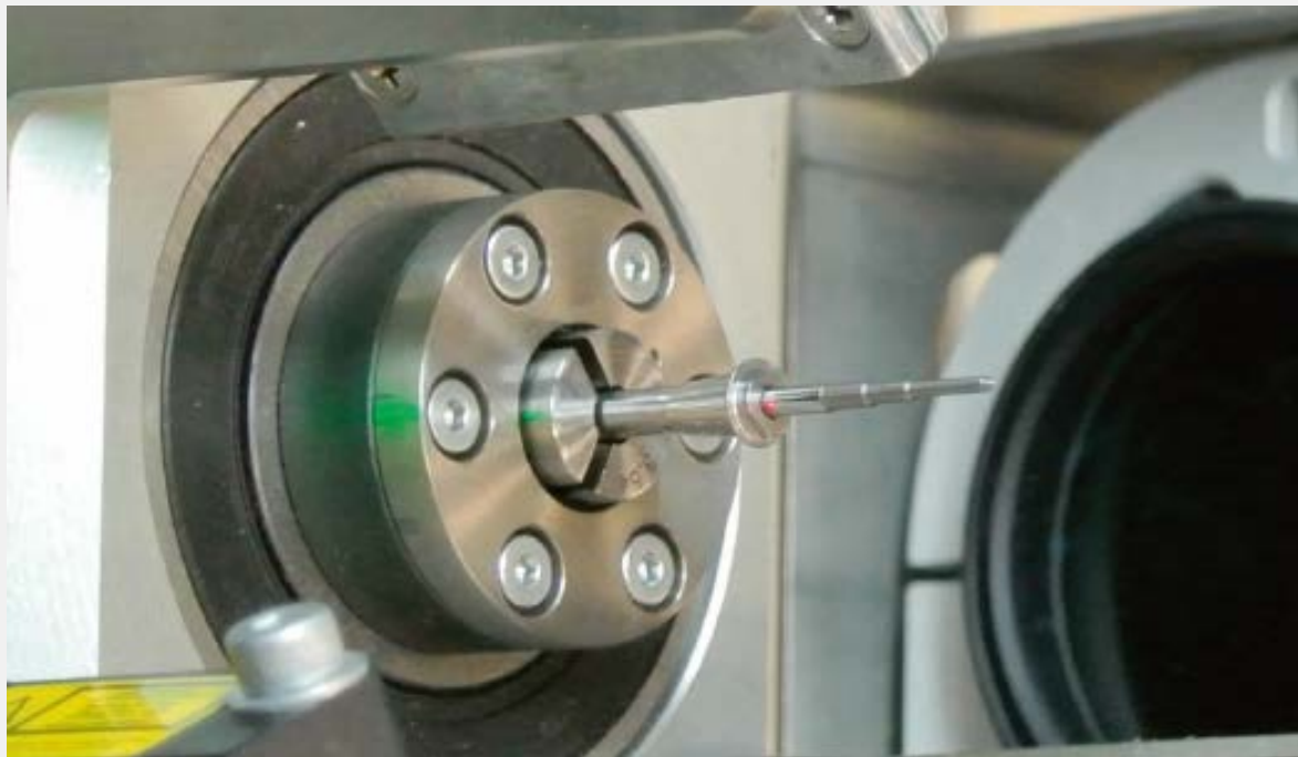
Part of the shaft runout test facility (Compar)
