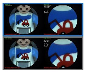
The blue print is shifted and distorted. However, this does not affect the human perception. Our print control (blue frame) is capable of accepting these non-disturbing variations and can still find the actual defects. Common softwares cannot do this (gray frame). (Picture: Compar)
