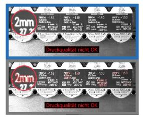
The slight distortion in the print is not disturbing to the human eye. Print inspection software without distortion compensation (gray frame) will, however, always produce false rejects without identifying the actual defects. Compar's Print Inspection offsets the distortion (blue frame). (Photo: Compar)
