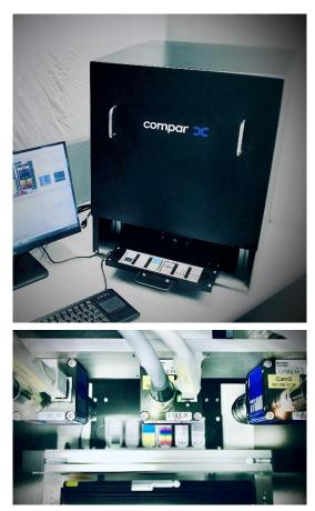
Example of a unit manufactured by Compar for separate quality control in the laboratory. Inside are three camera systems arranged in parallel (Photo: Compar)
