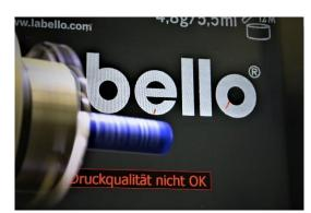
Analysis of the circular print on a rotating lip balm with the use of the camera above. Defects in the letters "e" and "o" are color-coded. (Photo: Compar)
