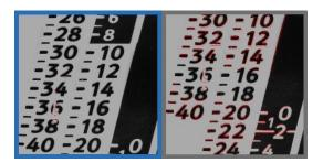
While real character defects (blue frame on the left) have to be recognized, the software can tolerate the "accordion distortions" of the circular print (gray frame on the right) in a parameter-controlled manner (picture: Compar)
